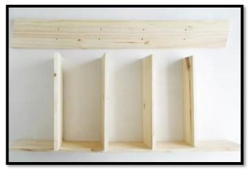
7. Repeat this last step screwing each shelf into place along the longer wood. Once one long side is completely done, repeat the previous step to attach the second side of the ladder with screws.
